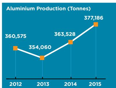
To achieve this feat, all departments across the smelter operated at significantly better levels than in previous years. The plant also achieved its best specific energy efficiency in the last 5 years at 13.7 kWhrs/kg. With the completion of the AP 39 lining, the plant is well on its way to operate at around 400kA efficiently. Metal purity levels improved significantly through the year contributing to outstanding customer satisfaction.
